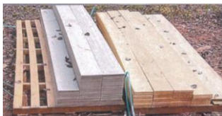
Neatly stacked on stickers, forklift-accessible
